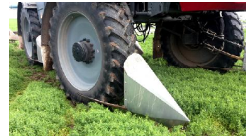
New crop dividers to minimise wheel track damage
