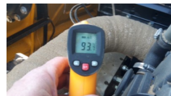
Testing exhaust temperatures in the lentils to prevent fires
