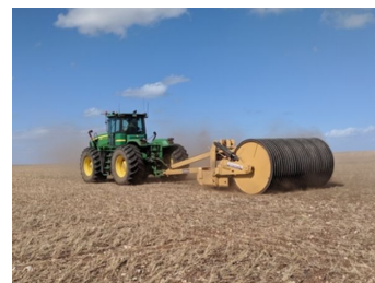
Reefinator ripping up limestone reefs at Ardrossan
